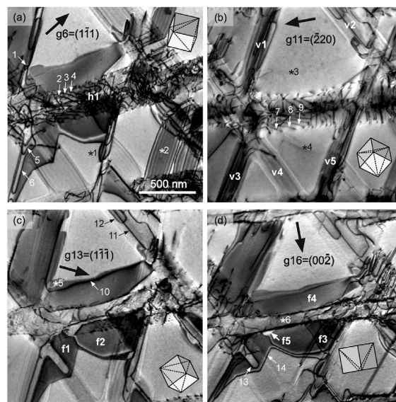
Advanced STEM analysis of dislocations and planar faults after 1% tensile creep strain accumulated in SX at 750°C and 800 MPa [C1_2].
