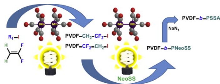
Figure. 1 Scheme of the \text{Mn}_2(\text{CO})_{10} -photomediated activation of perfluoro alkyl iodides under visible light in the initiation of the polymerization of NeoSS and VDF.
