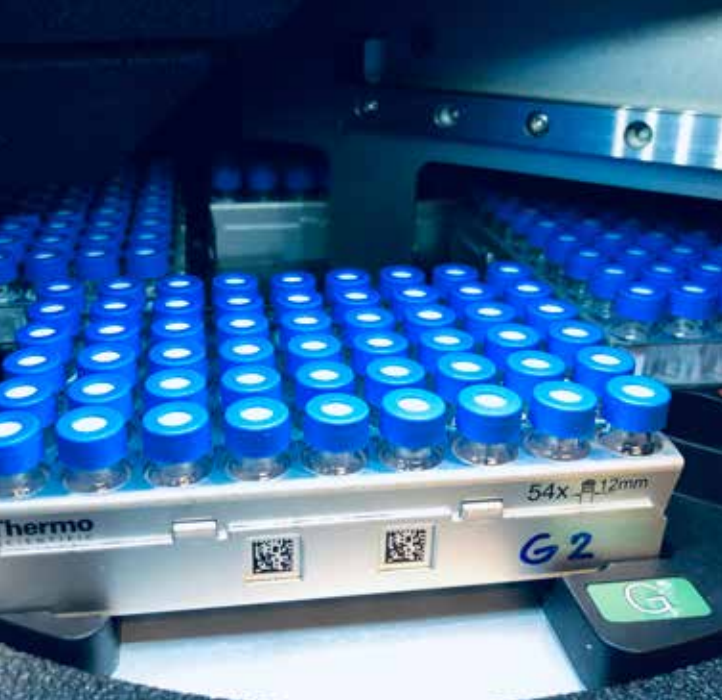
Automatic sample dispenser (autosampler), which is part of the liquid chromatograph assembly and mass spectrometer (LC-MS) for organic compound analyses
