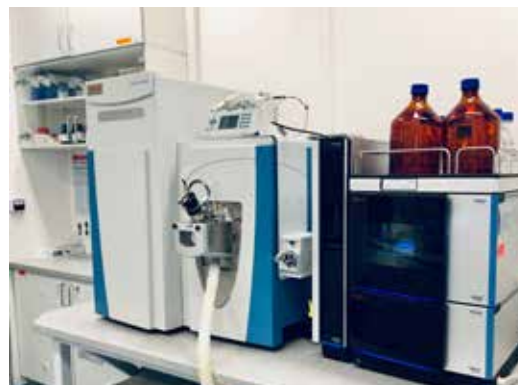
Automatic sample dispenser (autosampler), which is part of the liquid chromatograph assembly and mass spectrometer (LC-MS) for organic compound analyses
